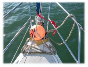
bow chain. Attach this chain to the bow ring below the anchor roller with a heavy stainless-steel carabiner. This chain is designed to take the load before the bridle in order to minimize chaffing.
